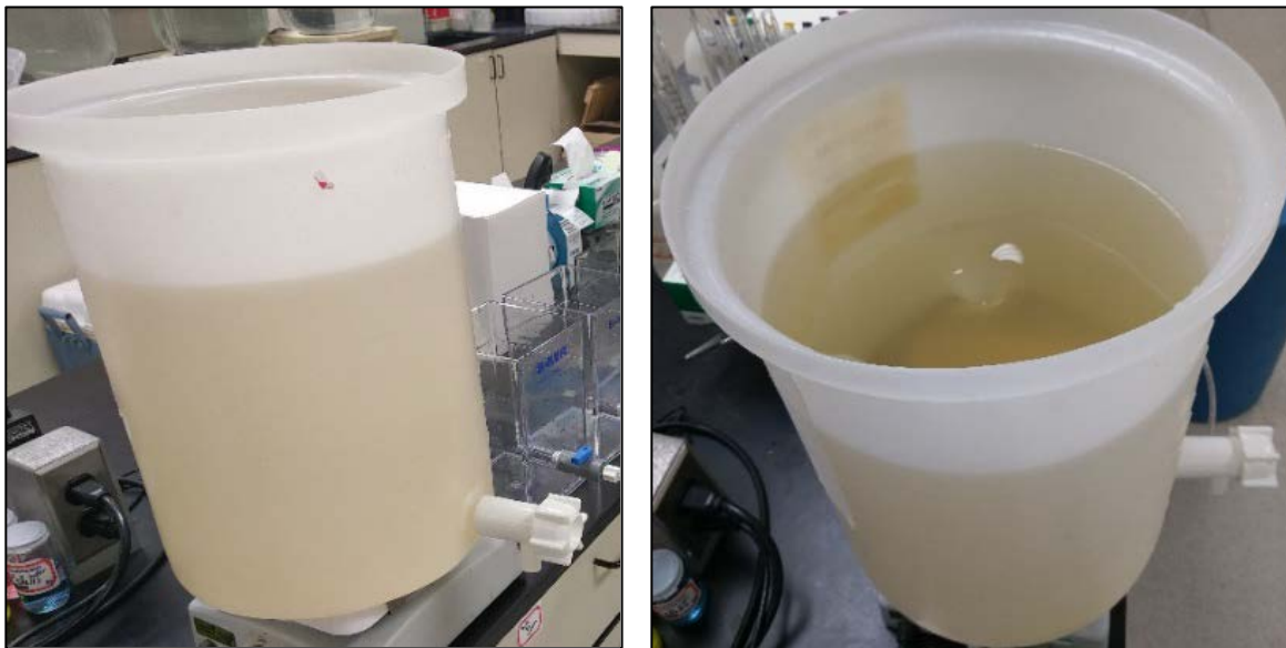
Figure 4-8: Raw Water Mixing Setup
