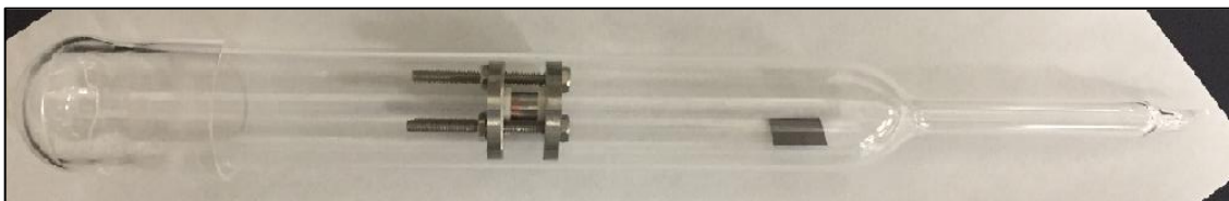
Figure 8 - Quartz capsule for encapsulation of diffusion couple under vacuum or inert atmosphere to prevent oxidation during high temperature anneal.
