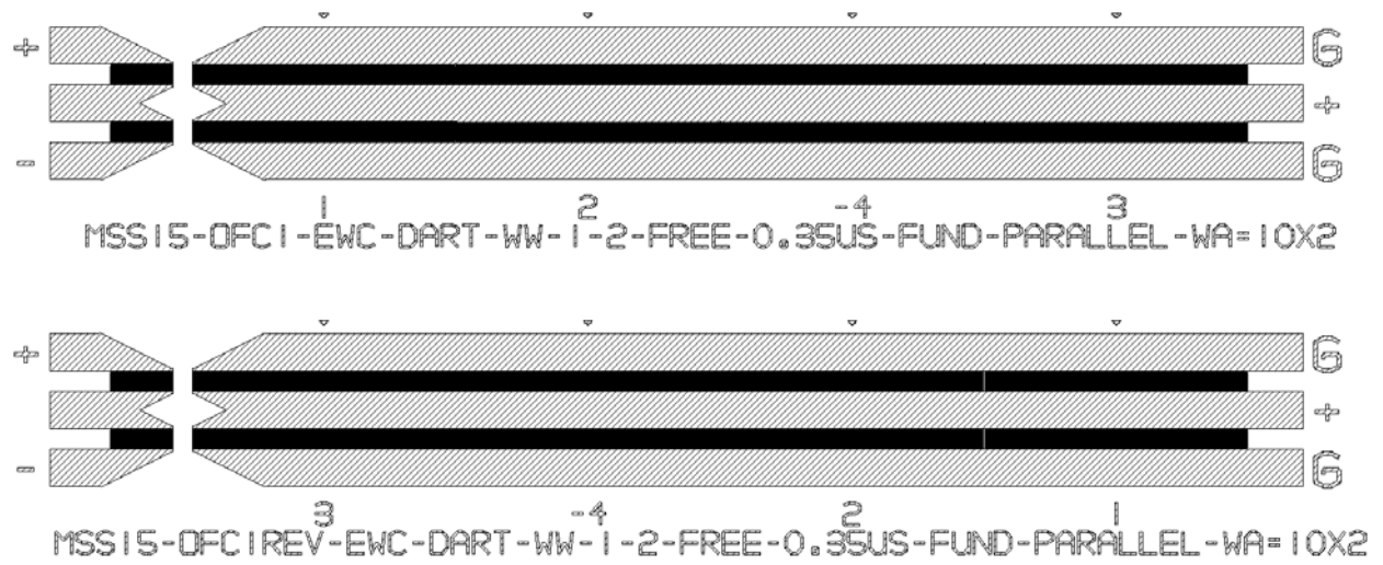
Figure 3.12: Device layout for final low loss OFC correlator filter matched code pair, with a forward code of [1,2,-4,3] (top) and reverse code of [3,-4,2,1] (bottom). On the left is the dual-track differential wideband transducer and on the right is the coded OFC transducer with single-ended parallel tracks. The large rectangles are bus bars and they are tapered at the ends in an attempt to reduce electromagnetic feedthrough, the dark area between bus bars are the electrodes which are too small to resolve. The full design is detailed in Table 3.3.
