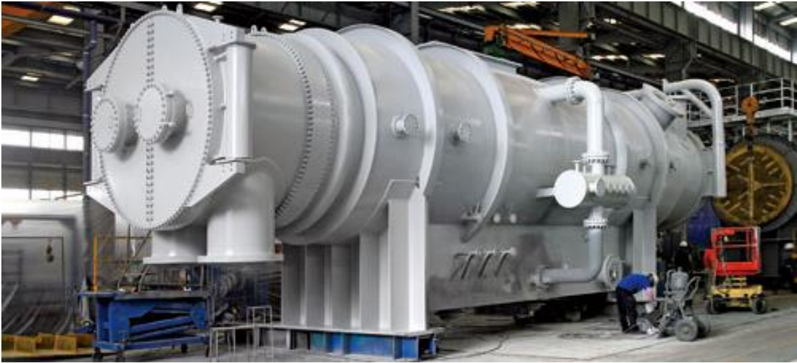
Figure 2.11: Combined-cycle power plant surface condenser
