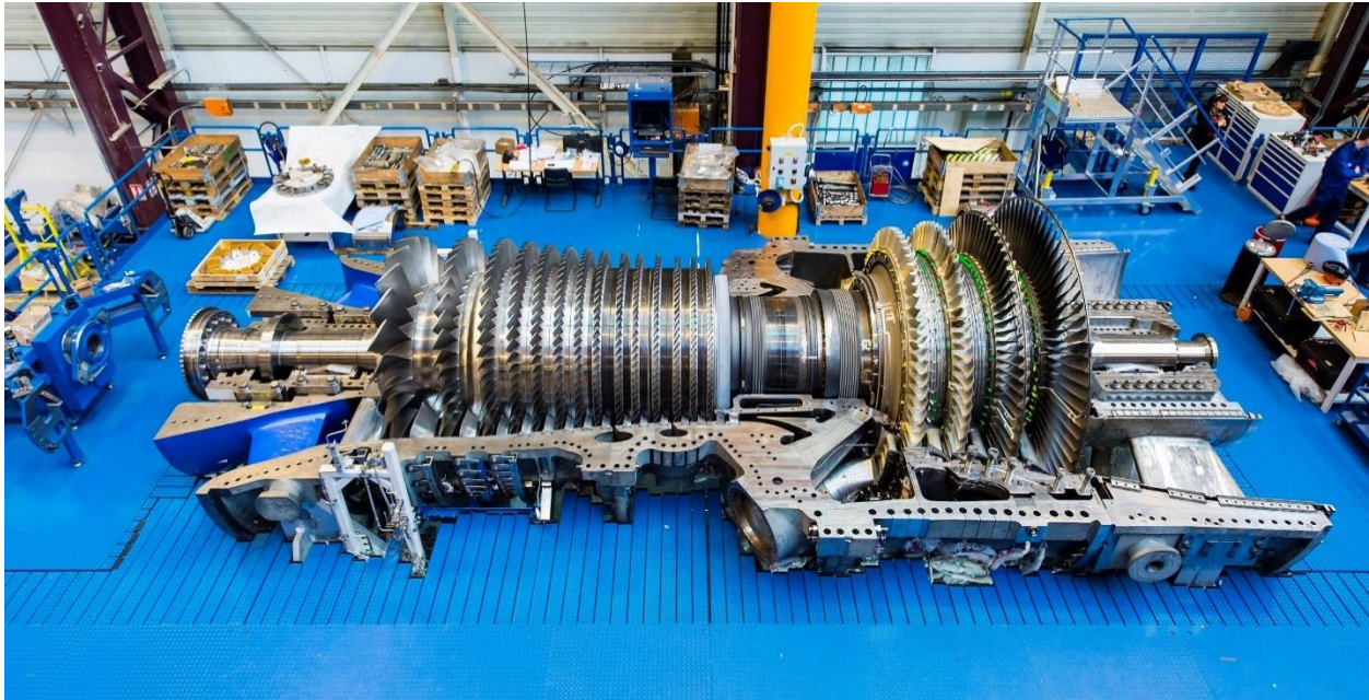
Figure 2.4: Assembly of a gas turbine rotor and casing
