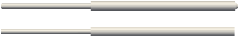
Figure 53: Computational domain with exit sonic nozzle (top) and truncated domain with exit nozzle removed (bottom)
