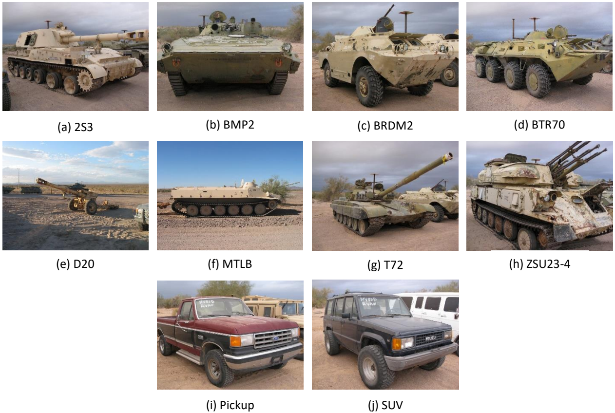
Figure 2 - Target data types from the SENSIAC ATR Algorithm Development Image Database [24]. (a) Self-propelled howitzer, (b) Armoured personnel carrier, (c) Infantry scout vehicle, (d) Armoured personnel carrier, (e) Towed howitzer, (f) Armoured reconnaissance vehicle, (g) Main battle tank, (h) Anti-aircraft weapon, (i) Civilian pickup truck, and (j) Civilian sport utility vehicle.
