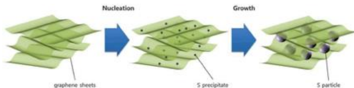
Figure 2- 23 Schematic diagram of heterogeneous sulfur crystal growth mechanism [62].
