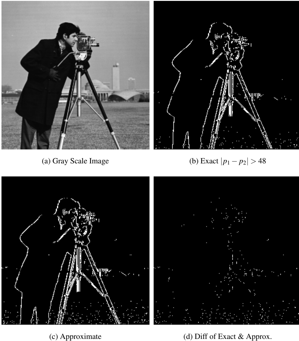
Figure 6.12: Comparison of our exact and approximate edge detection kernel on cameraman-image (a) is the original image. (b) shows result of approximate edge-detection kernel for \tau = 48 . (c) is the edge detection for exact edge-detection kernel. (d) is the difference between exact and approximate kernels. (e) is the overall error locations. Our design of approximate edge-detector is 28% more compact as compared to exact designs for only a 4% loss in accuracy
